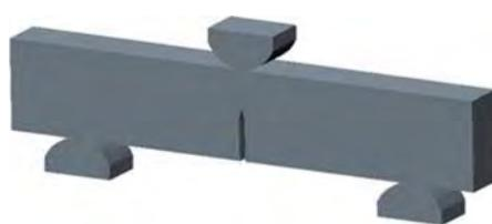
**Fig. 4** Geometric model for fracture analysis according to ASTM E1290
