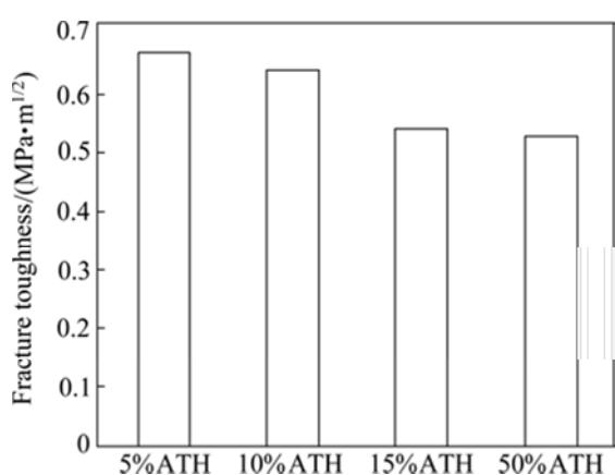
**Fig. 15** Variation of fracture toughness with different contents of ATH in PP/ATH composite
