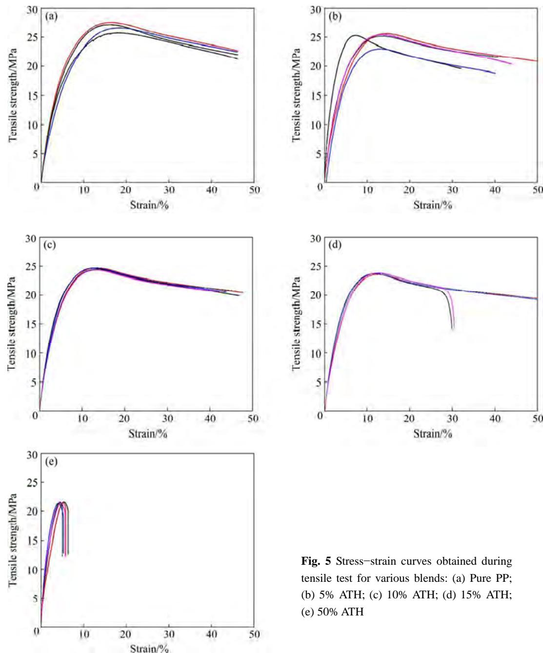
**Fig. 5** Stress-strain curves obtained during tensile test for various blends: (a) Pure PP; (b) 5% ATH; (c) 10% ATH; (d) 15% ATH; (e) 50% ATH
