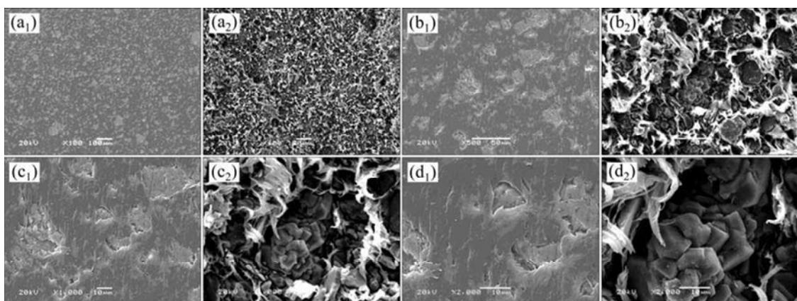
**Fig. 11** SEM images of fracture (50% ATH) specimen before loading (a<sub>1</sub>, b<sub>1</sub>, c<sub>1</sub>, d<sub>1</sub>) and after fracture (a<sub>2</sub>, b<sub>2</sub>, c<sub>2</sub>, d<sub>2</sub>): (a<sub>1</sub>, a<sub>2</sub>) 100x resolution; (b<sub>1</sub>, b<sub>2</sub>) 500x resolution; (c<sub>1</sub>, c<sub>2</sub>) 1000x resolution; (d<sub>1</sub>, d<sub>2</sub>) 2000x resolution
