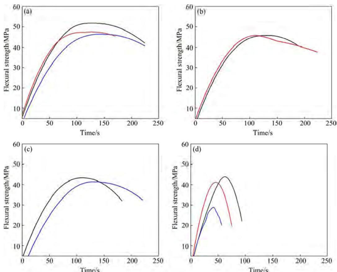
**Fig. 7** Flexural strength vs time plot for various blends of PP/ATH composite: (a) 5% ATH; (b) 10% ATH; (c) 15% ATH; (d) 50% ATH
