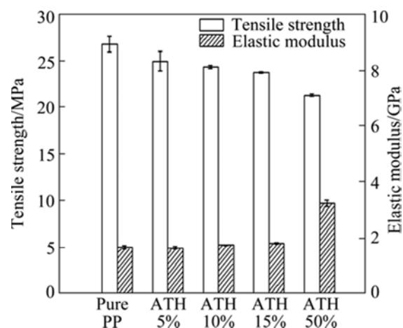
**Fig. 6** Variation in tensile strength and elastic modulus among different blends of PP/ATH
