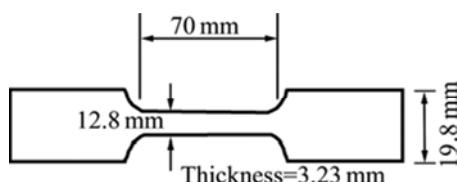
**Fig. 2** Dog-bone specimen for tensile test
