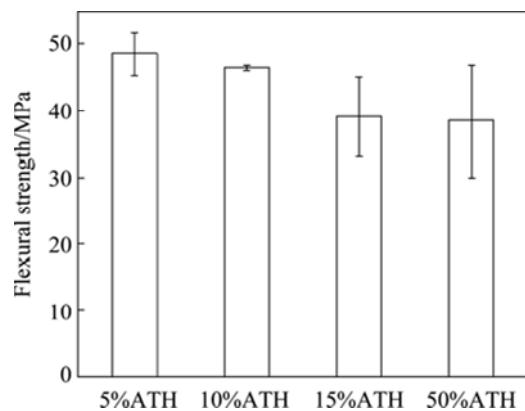
**Fig. 8** Variation in flexural strength of different blends of PP/ATH
