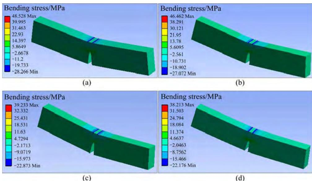
**Fig. 14** FE plots of bending stress in SENB of PP/ATH composite of different blends: (a) 5% ATH; (b) 10% ATH; (c) 15% ATH; (d) 50% ATH
