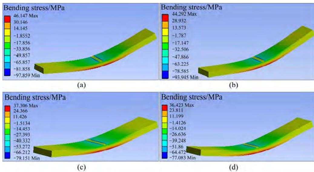
**Fig. 12** FE plots of bending stress in PP/ATH composite of different blends: (a) 5% ATH; (b) 10% ATH; (c) 15% ATH; (d) 50% ATH
